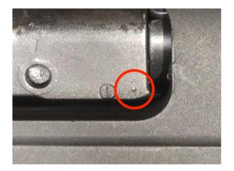
Remington has also corrected the manufacturing process to eliminate this potential firing pin problem in shotguns manufactured after November 24, 2014. Shotguns manufactured after November 24, 2014 will also have a punch mark on the bolt.
