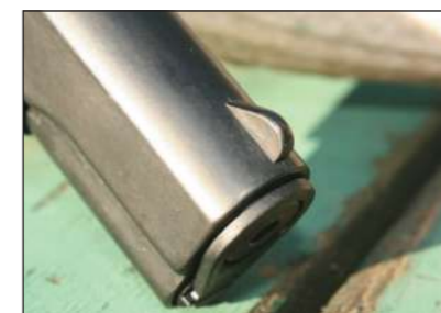
The front sight is a blade that is actually part of the slide; it is designed to be gently filed down in order to raise the point of impact in the event the pistol shoots too low.
