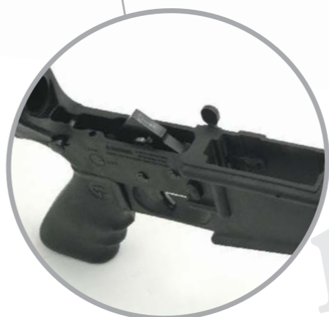
The lower receiver is made of high strength polymer, while the parts making up the trigger mechanism are made of steel, properly polished and hardened.
