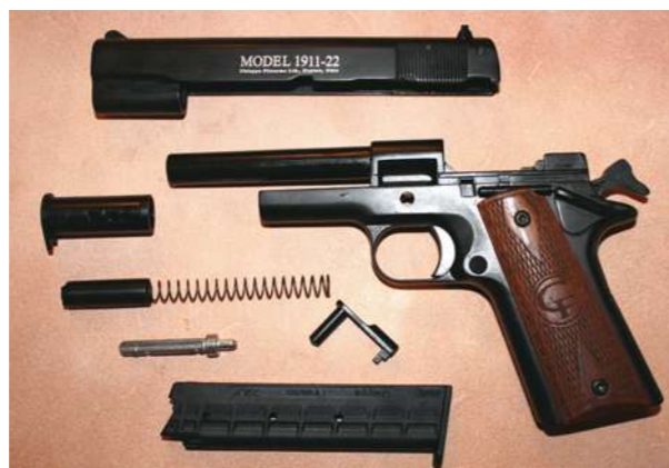
While the pistol looks like a Model 1911, it does not strip down like one. The barrel is fixed to the frame, and the slide must be pulled to the rear, raised off the rails and then pushed forward.
