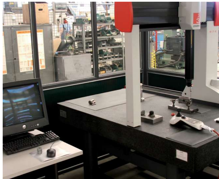
3-D machine to verify parts dimensions during production.
