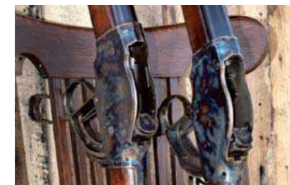
The original design by John Browning had been well conceived, but it left a couple of things to chance. There was no safety, and the semi-concealed hammer did not project much above the breech-bolt, making it tricky to thumb drop safely onto a loaded chamber. In that respect little has changed due to Chiappa's stringent desire for authenticity and the same rules of handling apply. The gun at left is a real 1887 Winchester.
