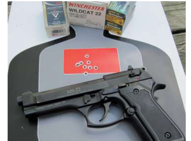
Unsupported 50 foot groups showed the Chiappa M9-22 is capable of excellent accuracy.
