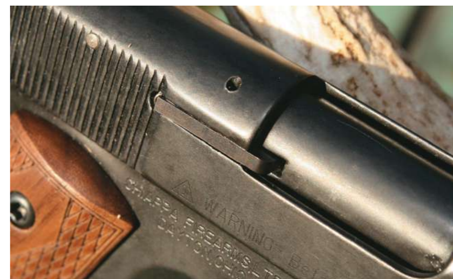
Chiappa designed this pistol with an external extractor that could double as a loaded chamber indicator if one looks closely.
