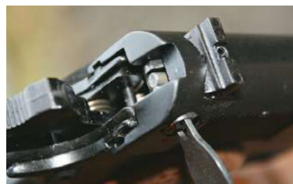
There's a manually engaged firing pin block safety in the slide that is turned into the "safe" position with a small two-pronged key that comes with the pistol.
