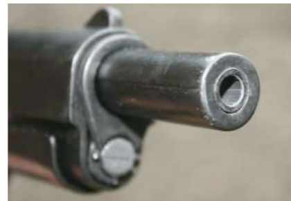
The non-ferrous alloy barrel has a steel tube insert, and this provides plenty of weight forward, which steadies the pistol and helps keep it on target.
