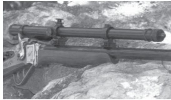
The Lyman tang sight and globe front sight certainly fit this rifle. To bring out even better results, the William Malcolm 3x scope is a good match to the gun's vintage lines.
