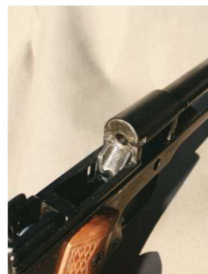
The fixed barrel has an integral feed ramp, and Workman found that the pistol functioned very well with all kinds of .22 Long Rifle ammunition.
