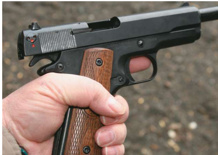
Also, just like John Moses Browning designed the original, the Chiappa's slide locks open after the last shot.
