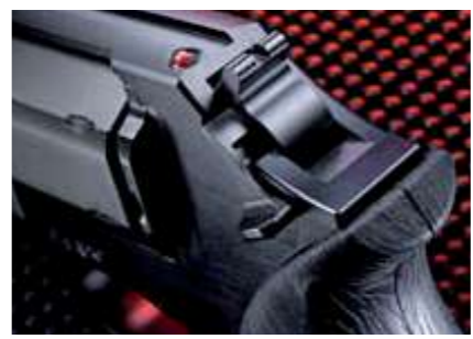
A red "cocking indicator" on the top of the Rhino lets the shooter know when it is cocked.
