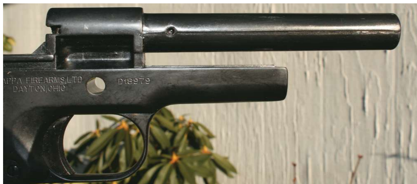
The fixed barrel contributes to the pistol's accuracy, which Workman found to be good enough to hit a tin can at 25 yards.
