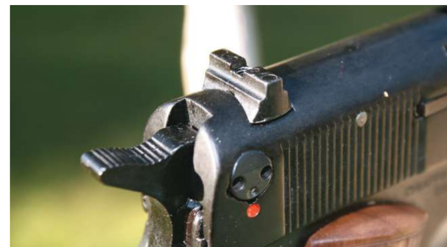
The rear sight is dovetailed into the slide and held in place by a tiny slotted screw.
