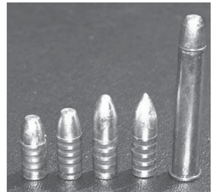
The Lyman Ideal Sharps’s 1-in-18” twist rate stabilizes bullets in the 240- gr. to 290-gr. range well, although it has trouble with longer bullets in the 310-gr. to 330-gr. range.
