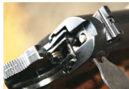
Turn the key back the other direction, and the block pivots down and out of the way, exposing the firing pin for a solid strike by the hammer.
